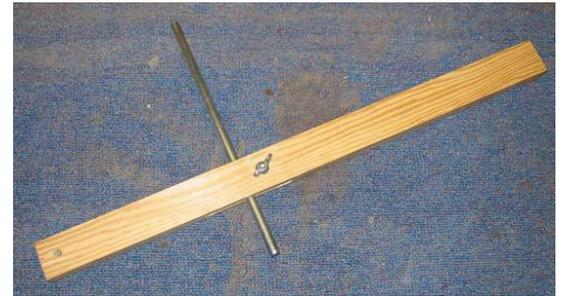
In use, the long side is placed across the bowl rim; the rod is positioned to the desired depth by sighting along the bottom of the rod. Then move the jig so that the rod is on the inside. This will tell you how much more wood can be safely removed. Remember to true up the rim before taking this measurement and, if you take any more cuts on the rim, be sure to reset the rod.
