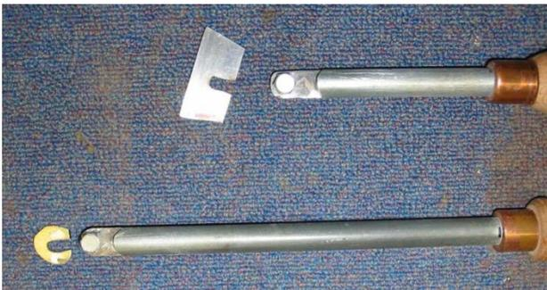
The second scraper shown is useful for the inside of a bowl. Therefore it needs to have a long reach, 10" out of the handle. The handle needs to be long for good control – in this case 19". The scraper itself was ground from a shaper blade
