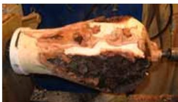
the faceplate. I chose the faceplate over a four jaw chuck because the overall length was going to 12+ inches. I used a 4in faceplate with 15-1 ½ #14 hex head screws (the largest that fit the holes in the plate). This put 1 inch of thread of each screw into the wood. You don't want this thing to vibrate or come off.
