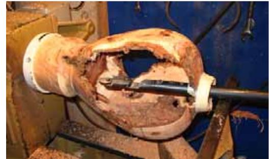
**Tip:** Fill small cracks with sanding dust (I use walnut because it is dark) then apply thin CA glue. The glue will swell the dust and lock the crack. The resulting seam looks like it belongs there.
