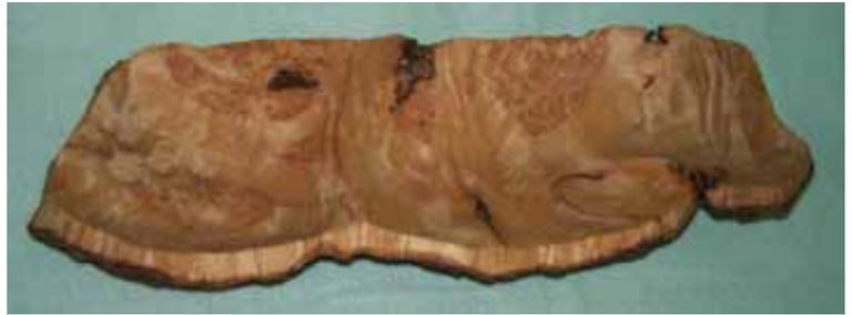
Alan usually textures outside edges off the lathe. He can use many styles of carvers to yield whatever textures he desires – rotary burs, hammer and punch, chain saw, air hammer and other tools to cut, depress, and crush to create a texture. Based on the lines Alan drew, he now knows where the cutout for the bowl needs to be. Then he hollowed out the bowl to the shape he desired.
