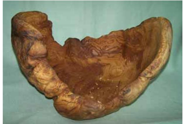
When the desire is to have the outside edge slanted on a burl, start the slant once you have solid wood all the way around the edge (no voids). This gives a more pleasing effect. A point to note ...the more design and texture on the outside irregular edge of a bowl, the more difficult it is to sand.
