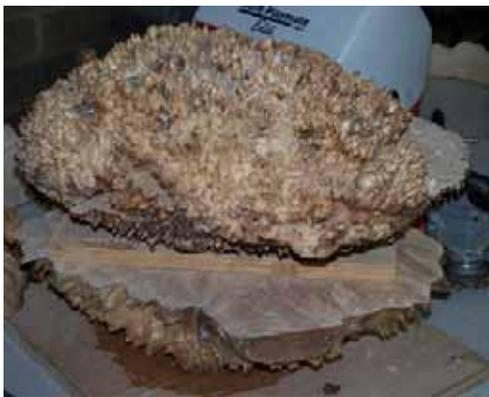
Be careful to use calipers to avoid going thru the bottom (a laser is even better). When you use really wet wood, check the chuck often as the burl may shrink as you turn, especially if it is on the lathe a long time. Alan removed the tailstock and then proceeded to finish hollowing the center.
