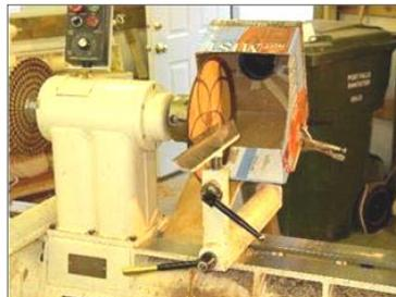
I started with a packing box so I could "cut and fit" while I tried to find a way to install a more permanent collection hood that would still give me access for turning and sanding. In the end, the permanent solution was to find a better box. If I want a larger hood, I get a larger box.
