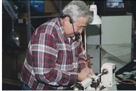
progressively. Be careful and cautious! With the blanks spinning a little sanding goes a long way. When you have finished sanding with 320 grit sandpaper, brush the blanks with a mixture of 1 part lacquer sanding sealer, 1 part high gloss lacquer, and 1 part lacquer thinner. Then with the lathe running, wipe off this mixture with a paper towel. The blanks are now sealed and you can continue to sand up to 600-800 grit if necessary.
