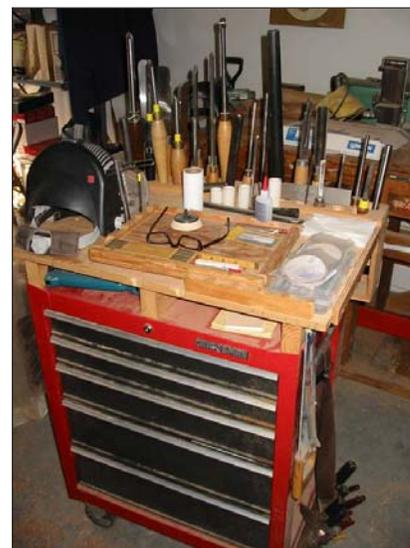
Don's sharpening system consists of a 6-inch grinder situated atop a stand made of 4-inch PVC drain pipe equipped with fittings for the wooden base and a platform for the grinder. Since he doesn't like to bend over to sharpen, the stand brings the grinder to shoulder-level. He uses a homemade knockoff of the Wolverine system, though he did buy the Vari-grind attachment.
