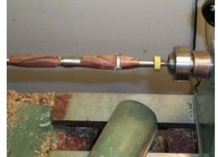
iron. Mine was okay. Return the work to the lathe and turn down the ring to match the surrounding surface. I took very light cuts with a freshly sharpened spindle gouge, followed by a skew.
