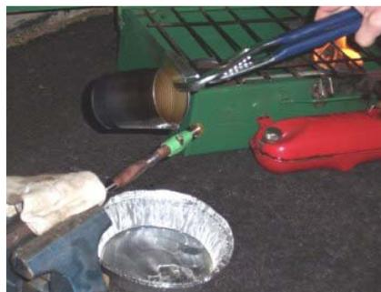
spilled pewter (once cooled) can be tossed back in the melting pot for next time. Pour quickly and carefully. Try to hit one side of the hole in the tape so that the metal flows around and up to the other side. Now you can shut off the heat and let everything cool down.
