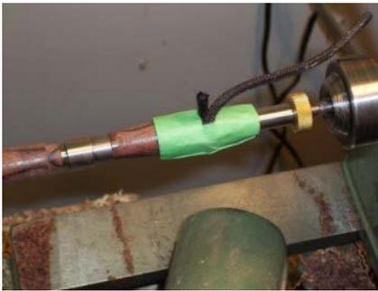
Now carefully withdraw the cord, leaving a ring-shaped cavity under the tape, and a hole where you can pour in the molten metal. Scott said he sometimes makes a
