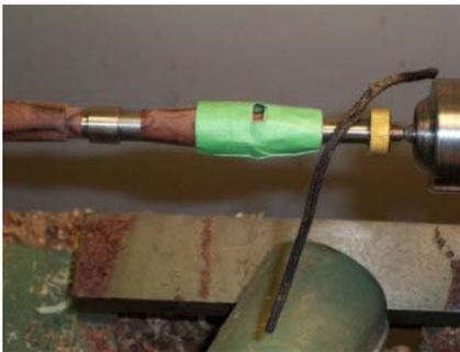
cone from masking tape and adds some plaster of Paris around the opening to support the cone. This enables you to get some pressure in the mold so it fills the cavities better. My ring was so small I decided not to use anything more than just the tape.
