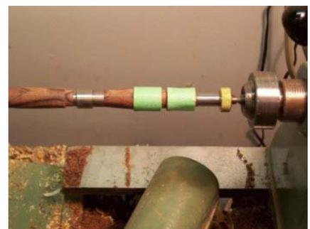
I put four layers of tape on either side of the groove. Burnish it well, so it sticks. You don't want the tape coming loose and spilling metal all over the place. Then you lay in some waxed or greased cord to fill the groove and to make the tape retain some shape when you burnish it. I used a piece of an old shoe lace coated with paste wax. The wax is to keep the tape from sticking to the cord.
