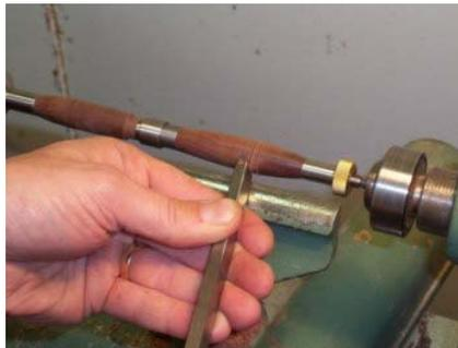
Follow up with a parting tool to clear the waste. I went about 3/32" deep or perhaps a bit more. On a pen you don't have a lot of material to work with so I left this part of the pen rather fat. In retrospect I could have made the pen narrower at this point, and the groove shallower, and the pen would have had a more sleek look.
