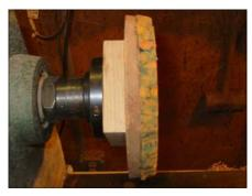
I use a dedicated screw chuck but all 4 jaw chucks come with a screw center. Now put the open end of the bowl over the pad and position the live center into the center hole left from the rough turning. Turn the tenon round and face off a flat. Now is also a good time to decide the shape of the bottom and do the preliminary cutting while it's on the pad.
