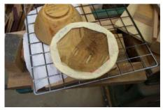
these cases the roughed out wall the paper over the rim, trim off the thickness needs to be thick enough to excess, and place the bowl upside down will completely prevent movement of foot it may not rest evenly due to the the wood when it dries, so plan your paper and the air may not circulate as well. The inside of the bowl needs to be exposed to air.
