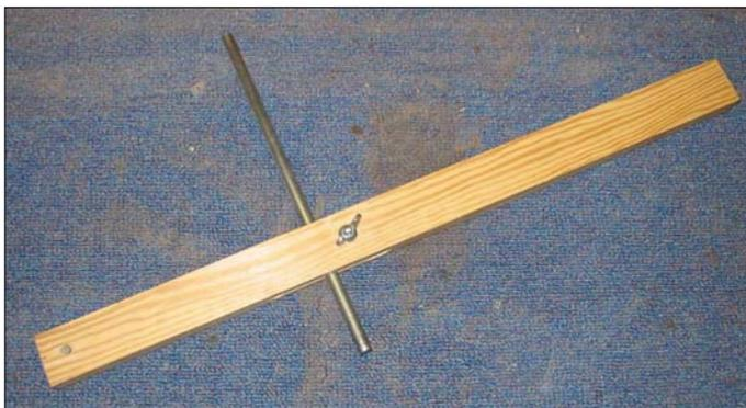
that there is wood 8" on one side and at least 14" on the other. These dimensions are for use with a 16" swing lathe. Buy a piece of 1/4" curtain rod about 10" long. Using a saber saw cut out some wood about 2" on either side of the hole. This will allow the wood to flex holding the rod tightly in position when the thumbscrew is tightened. In use the long side is placed across the bowl rim, the
