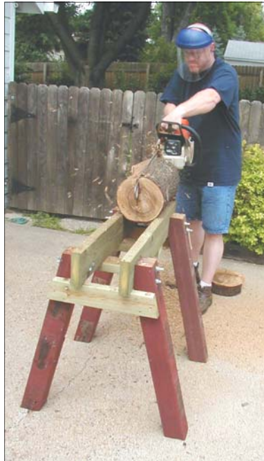
Steve sawed this bowl blank in half with the log held in place between the 2 x 6 uprights.
