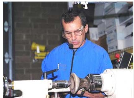
To order to learn to balance and bend the discs Steve began making metal coasters. As the discs became larger platters he learned to add beaded edges to provide stiffness. He has now progressed to vessels with multiple curves.
