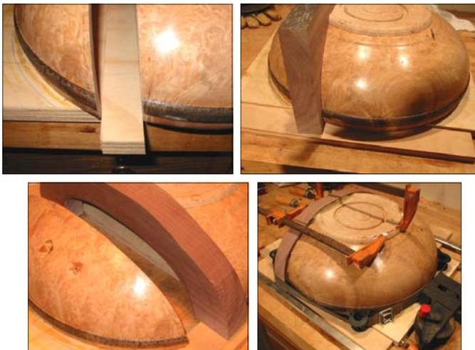
After the glue dried, I knocked off the base boards. Next, I used a combination of grinders and sanders to trim off most of the Walnut board. The bowl was then placed back on the lathe and re-turned. Less than an 1/8" of an inch had to be
