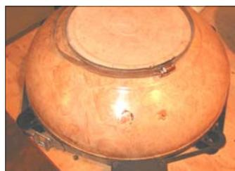
Once glued back together, I remounted the bowl on the lathe. First I cut a new groove in the bottom for the chuck to use during the next turning. The pictures show the laser light. I used the laser to highlight a straight line on either side of the outermost edges of the crack.
