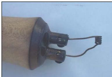
Here's a close-up of the pen tip and brand I'm using. This is the brand that gives me the basket weave pattern. It's just a 20 gauge nichrome wire that has been wound around a nail.
