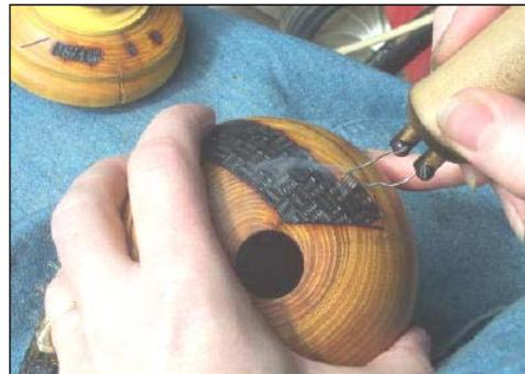
This photo shows how I always have a finger braced against the piece to steady my hand. It's kind of like an outrigger on a canoe, which provides balance and stability.
