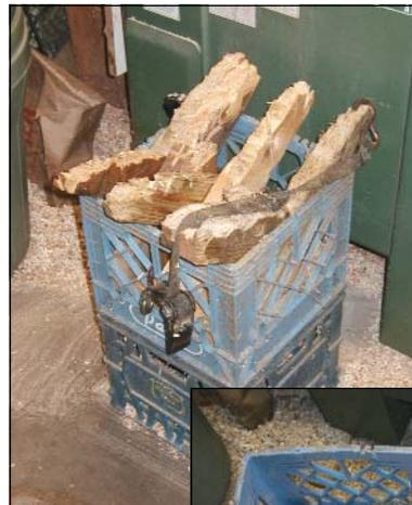
If you use an electric chainsaw in your small shop, this sawhorse is very useful and simple. Made from 2 milk crates, 2x4's and a wooden dowel. A nylon clamp can be used for a hold-down. Two 2x12's were put in the bottom for spacers.
