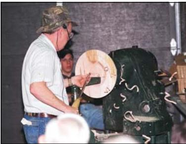
Terry turned a bowl in his style starting with the blank held on a faceplate (remember his lathe has no tailstock). The blank was trued using his cutting method of pulling or pushing the gouge from right to left with the flute pointing at
