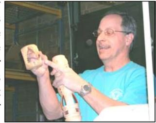
faster if you have a proper setup. To glue the blocks up, for turning the inside, John has used a paper glue joint, strapping tape, screws, and CA glue with accelerator. His favorite method by far is the paper glue joint. It is easy to break apart when he is ready to turn the outside and there is a low risk of the pieces coming apart while turning. He numbers the blanks and cuts the corners, when glued up for the inside turning, to ensure he puts it together properly for the outside turning.
