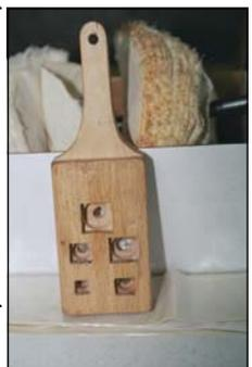
Before placing the blanks on the mandrel, you want to insure that the mandrel is straight so that you don't end up with an oval shaped pen. Greg held a pencil on the tool rest and very gently brought it forward until it barely made contact with the mandrel. If the line does not go all the way around the circumference, then the mandrel is not straight.
