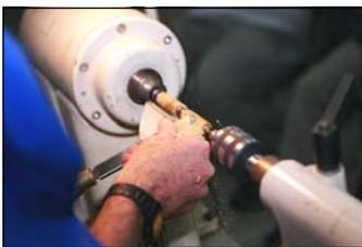
Greg's favorite tool is the skew. He has put a little curve on his grind because when he is finished turning there is little sanding involved. As you cut a pen it will typically have a slight taper. This taper needs to be kept consistent and Greg feels he has better control with the skew.
