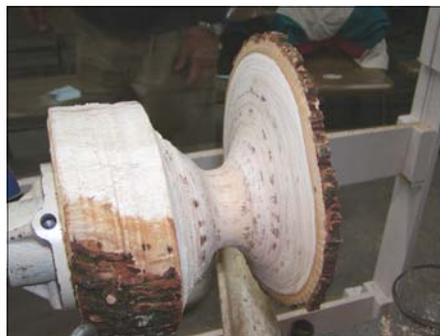
He begins by removing bark and wood from the center of the piece in a spindle manner. He then moves to the end grain and begins to remove wood from the interior of the log, he intends to retain the "natural edge" in the final piece. He continued to remove woodworking toward a 1/4" thickness. As he moved through the log he showed how the "soul of the tree" is exposed. I was impressed with the number of times Don stopped to check thickness or thinness of his work.
