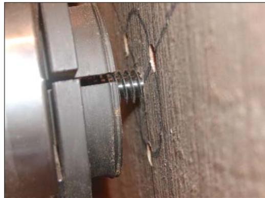
9. Rough turn bottom of the platter, and true up the edges. Keep the foot area oversized, say 8" diameter, and at least 1/4" thick.
