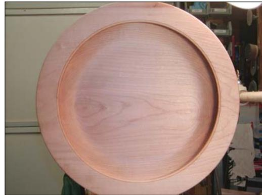
16. Remove platter from screw chuck, and re-mount in third off-center hole.
