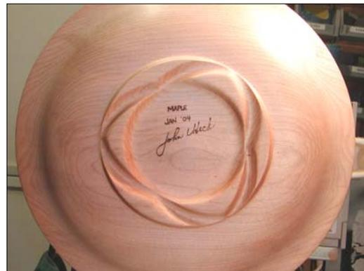
18. Remove platter from screw chuck, and re-mount in center hole.
