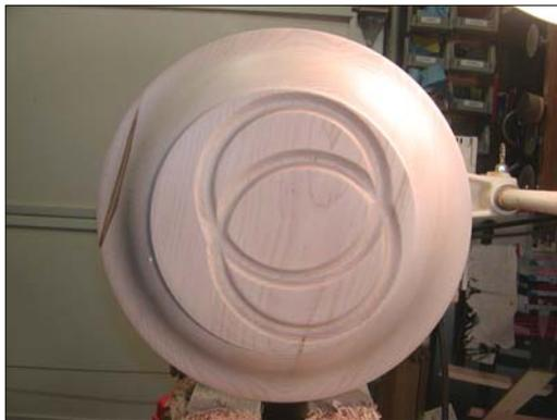
22. Remove the platter from the screw chuck, reverse, and mount on your chuck, clamping onto the tenon.
