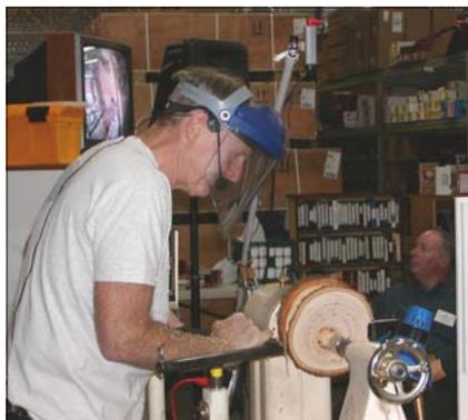
He demonstrated his personal tool supply including a boring bar used to hold 1/4" bits held in with a setscrew and a "stout" bowl gouge. He calls the boring bar with bit a Carpenter Ant Tool. He does bring up the tailstock to support the piece but he does not use the live center point to hold the wood. Don prefers a round tool rest as opposed to
