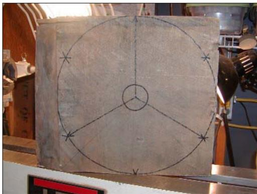
6. Drill a 3/8" hole, 1" deep (depending on your screw chuck), in the center, and at each of the three locations on the 1" center circle.
