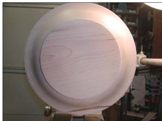
10. Remove platter from screw chuck, and re-mount in one of the off-center holes.
