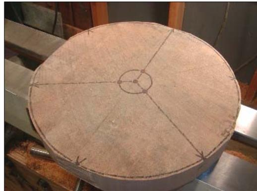
8. Mount the blank in the center hole using a screw center, then tighten it so it completely seats on the chuck jaws.
