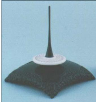
a 2" square piece of black wood 1/2" thick, and he turns a convex shape using the chuck and a point for the top to dance in, on one side, and then reverses the piece in the chuck, and turns a convex shape for the bottom and four points to stand on. Then he "stipples" around the edge of the piece for a pleasing effect.
