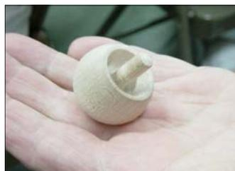
Use a fine cut here as you don’t want to sand the inside; round the sides, and come back and refine the outside shape with the 3/8” bowl gouge. Next sand 100 to 600 grit paper two coats of lacquer, and wax; part off with a butter knife parting tool, and ready for a spin. The rounded shape of the top begins spinning like a normal top, and as it slows, rights itself, and starts spinning on the stem of the top!
