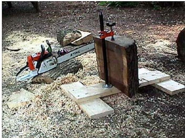
It is pretty easy to build and use. I bought a Pony clamp that slides along the pipe but also has a screw adjustment on it, a 24" length of 3/4" black pipe, a pipe flange, and an 8' 2x10. Assembly should be apparent, dimensions are not critical. To use it, place the blank on the jig, and clamp it down. It works quite well, and I have had a significant improvement in sawing out uniform bowl blanks.
