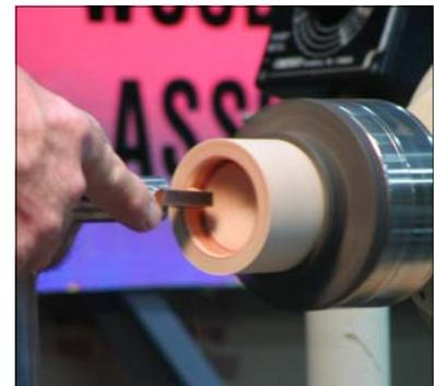
Touch the thread chaser to the edge of the wood to "strike" a thread, get into a rhythm to start a pattern, add Joy magic, make the thread a bit deeper and carefully add pressure to the arm brace cutting a deeper thread each time. Cutting above center about 10 degrees. This is 20 threads per inch which he likes for his boxes.
