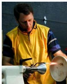
To finish the bottom of the bowl Ric uses a home made chuck that is a hybrid of a compression and Longworth chuck (see resources at the end of this review). The chuck gives him very unrestricted access to the bowl bottom. To center the bowl on the
