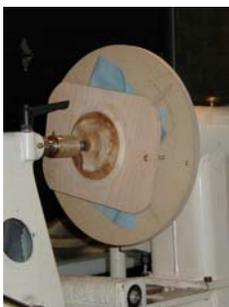
chuck he mounts the chuck on a tailstock chuck adapter in the tailstock. He then brings this assembly up to the bowl still mounted on the headstock and tightens it.
