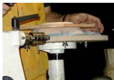
To carve the majority of the wood from around the feet Ric uses a Roto-Zip tool with a 1/4" burr cutter bit. He then uses power sanding pads and a palm sander to further refine the shape. To carve a fluted rim Ric follows similar steps which he thoroughly discusses in the video.
