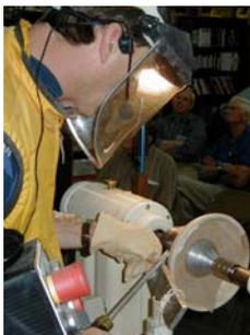
Next, he used a propane torch to light burn the outer rim and then used 20-gauge steel wire to further accent the rim with a fine burned line.
