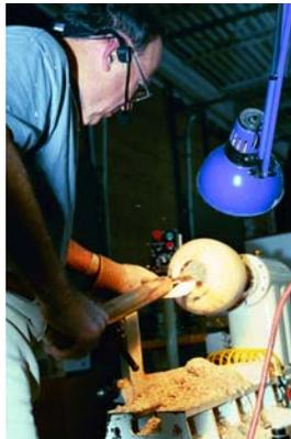
Knud's technique used 1/4" and 3/16" machine tool bits held in a variety of handled straight and angled steel rods. Although it is quite common to see commercial tools of this kind sold today, Knud was probably the first turner to make extensive use of this kind of tool. And now Darrell has his own line of these tools utilizing an outboard fork to counter the torque of the cut.
